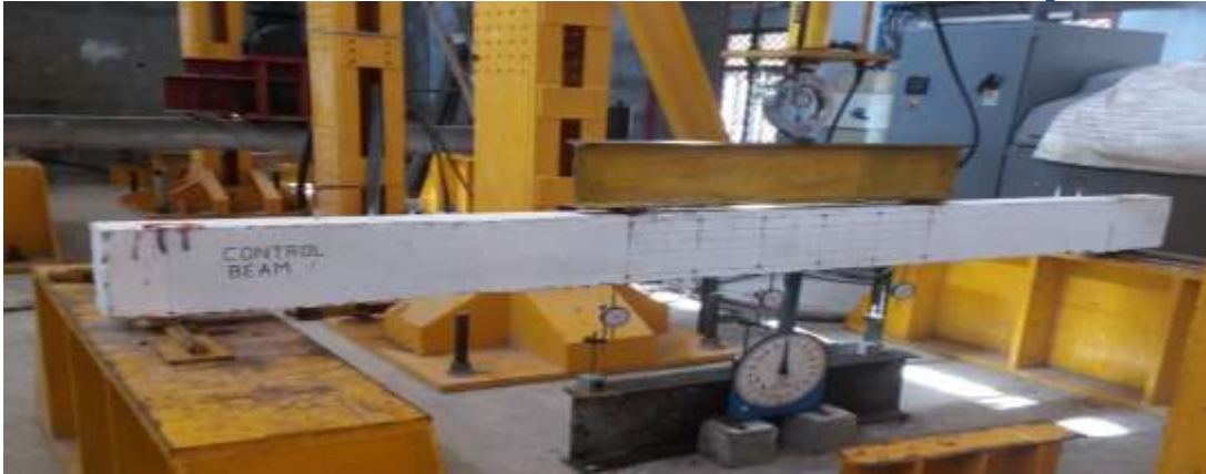
Figure 7 Testing of Beam
