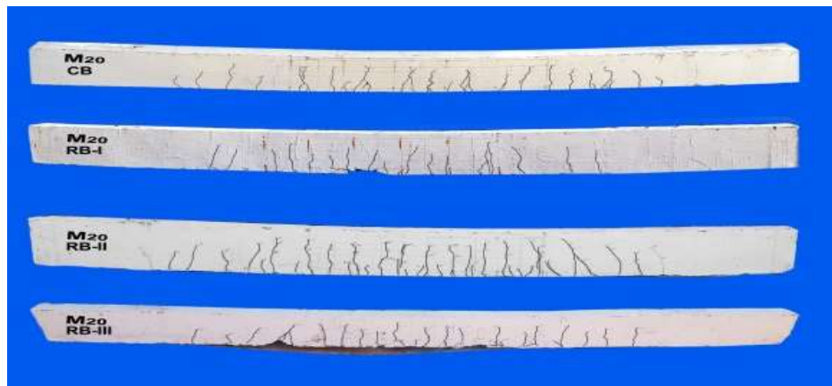
Figure 8 Control GFRP Sheet Strengthened RC Beams
